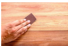
Fig. 10. A piece of sandpaper is made by affixing small bits of corundum to a thick strip of paper or cloth.
