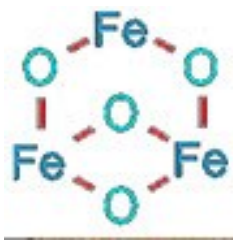
Fig. 13A. A molecule of magnetite consists of three iron atoms (Fe) bonded to four oxygen atoms (O), or \text{Fe}_3\text{O}_4 .
